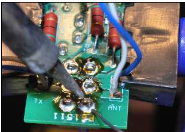
Soldering new switch in place
